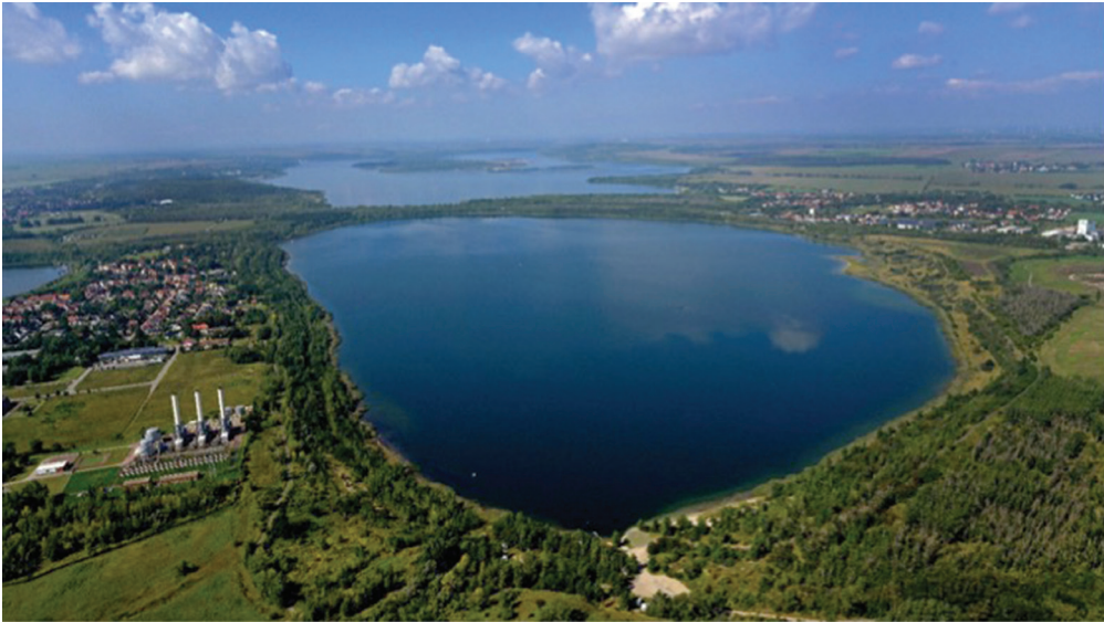
Figure 1 Pit Lake Runstedt with Pit Lake Geiseltalsee in background and the narrow overburden dam separating them (image: LMBV, 2019).
