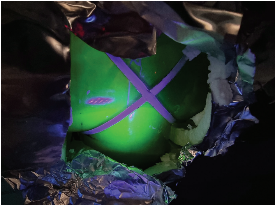
Figure 4 Tracer injection via a hose into shaft #4, accumulation of tracer in the shaft sump (experiment 2)
