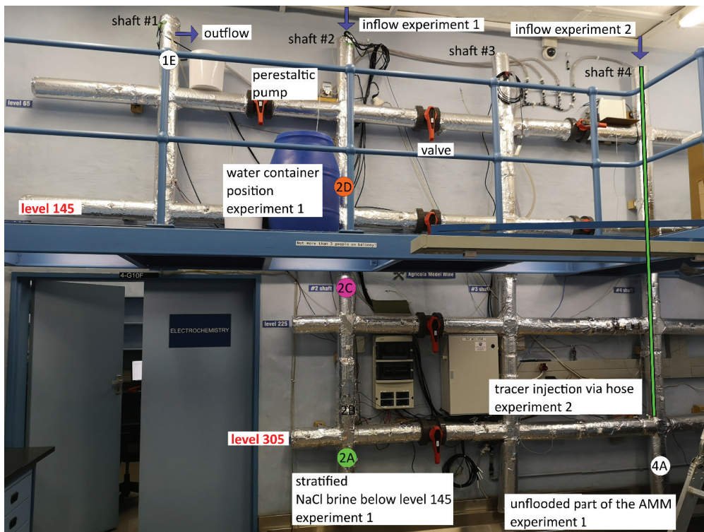
Figure 1 Agricola mine model (AMM) with water container and peristaltic pump position for experiment 1; in round circles selected injection and sampling ports; 2D (orange) injection EoY, 2C (pink) injection SRB, 2A (green) injection EoY; green hose in shaft #4 injection EoY above level 305
