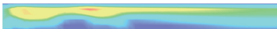
Figure 6 The velocity cloud atlas of the flow field in the later stage of aggregate accumulation
