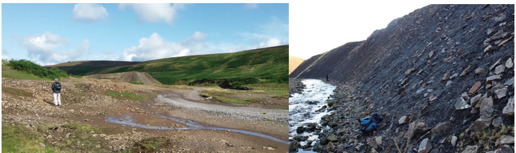
Figure 1 a Left: areas of investigation, looking north with drainage crossing the dressing floor in foreground and vegetation free driving spoil bund mid-distance. b Right: field sampling of the stream side of the driving spoil bund. Note range in grain size and seepage.
