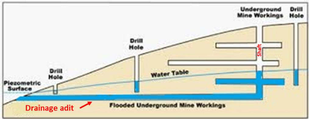
Figure 1. Schematic design of drainage adit (Source: adapted from Bourgeot et al., 2016).
