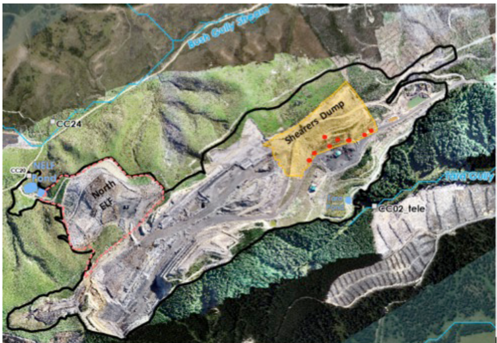
Figure 2. January 2018. Seepage sites associated with the historic Shearers Dump (red dots).
