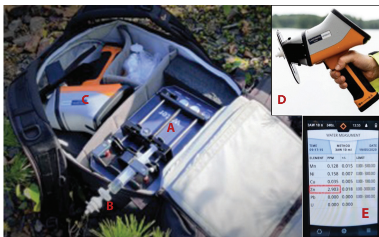
Figure 1 The 3A Water Multimetal Water Analysis System (MWAS, prototype 2.1): A) Battery operated syringe pump, B) consumable filters including a 0.45 \mu\text{m} prefilter and the metal collecting filter inside a filter holder, C) handheld XRF spectrometer, D) adapter on the spectrometer with the filter holder inserted and E) image of the screen of the spectrometer showing results from an on-site analysis (not specific to the present pilots).
