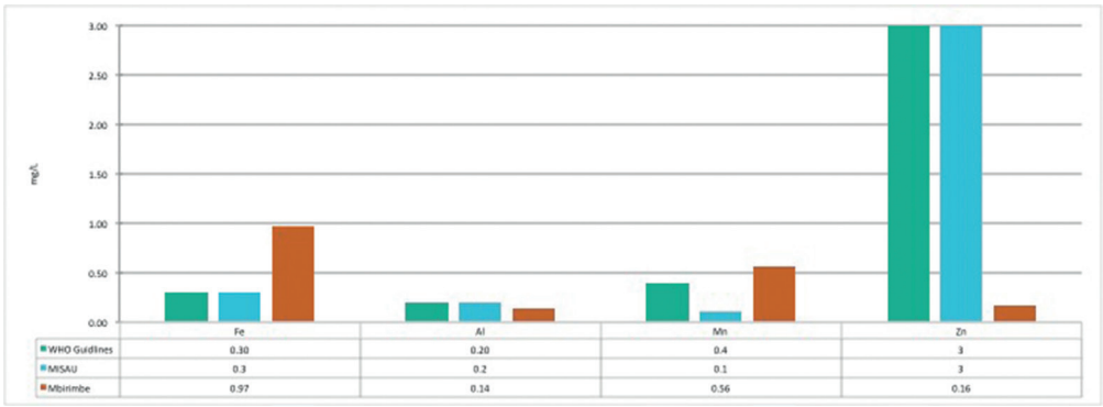
Figure 3 Observed metal concentrations in Mbirimbe River (red) in comparison with WHO-drinking water guidelines (green) and MISAU regulation (blue).
