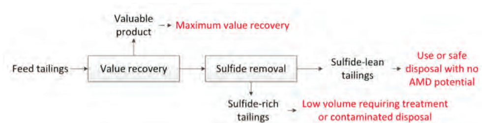
Figure 1 Two-stage separation process developed by UCT researchers (Hesketh et al. 2010; Kazadi Mbamba et al. 2012).
