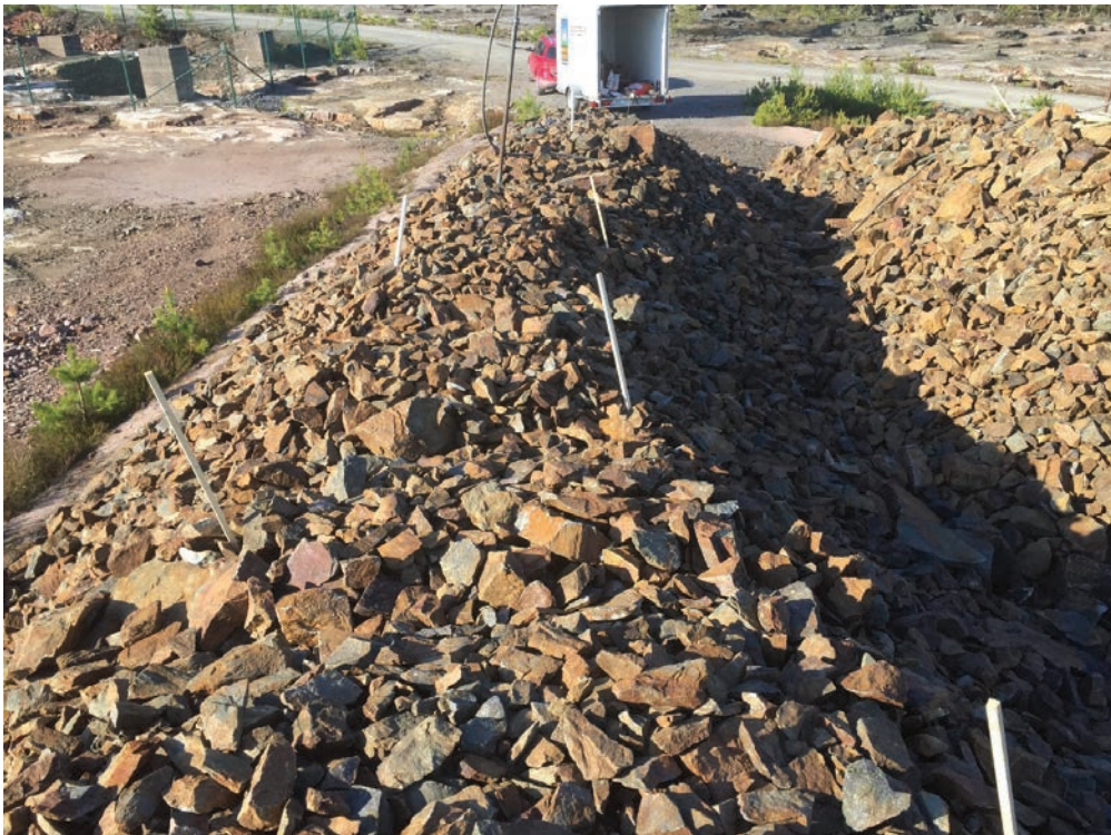
Figure 2 Part of the waste pile (parts of piles 3 and 4) and injection points marked.
