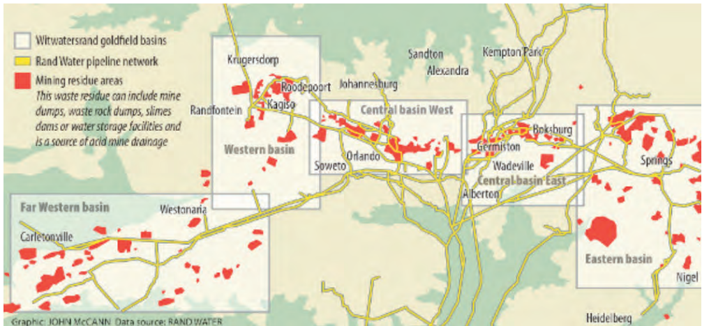
Figure 1 Rand water pipeline and proximity to mine waste dumps on the Witwatersrand. (Source John McCann).
