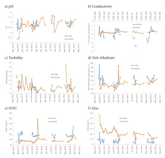
Figure 4 Physico-chemical parameters for the river inflow and outflow from Lake Kepwari (2013-2016).
