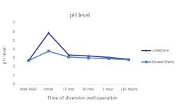
*Figure 6* Graph showing comparison of pH levels for limestone and mussel shell treatment.
