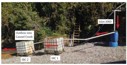
*Figure 3* Diversion well setup at Bellvue Mine site. Inlet AMD enters the well where fluidization of substrate occurs. Treated water then flows through each IBC, where further dissolution of substrate and neutralisation reactions occur. Treated water then flows into Cannel Creek.
