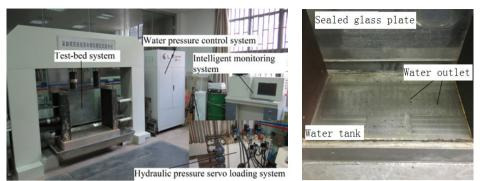
Fig. 1 Similar Simulation Experiment System for Water-inrush From the Mining coal seam floor Fig. 2 Water-tank Pad
