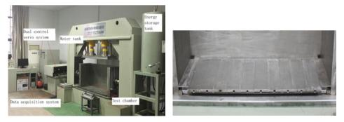
Fig.3 Roof water and sand inrush of mining simulation system Fig. 4 Coal seam drawing board
