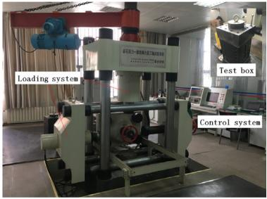
Fig. 5 True Triaxial Rock Test System of Coupled Stress-seepage
