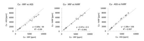
Figure 5 Comparative hXRF measurements on press tablets: XRF and AAS values – Cu content in copper mine tailing material (dashed line: regression line; dotted line: congruency)
