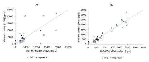
Figure 1 Comparative hXRF measurements: field-, cup- and chemical-analytical values – As and Pb content in zinc-gold mine tailing material (dotted line: congruency of chemical-analytical value and hXRF value)
