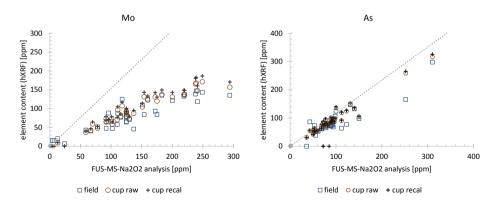
Figure 6 Comparative hXRF measurements: field-, cup- and chemical-analytical values – Mo and As content in copper mine tailing material (dotted line: congruency of chemical-analytical value and hXRF value)
