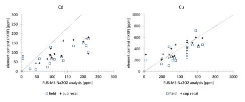
Figure 2 Comparative hXRF measurements: field-, cup- and chemical-analytical values – Cd and Cu content in zinc-gold mine tailing material (dotted line: congruency of chemicalanalytical value and hXRF value)
