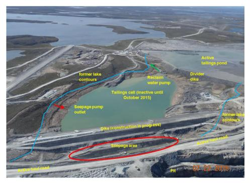
Figure 6 – Tailings facility seepage area site plan
