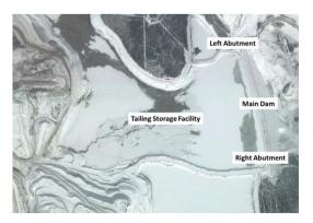
Figure 3 – Valley fill tailings storage facility and dam.
