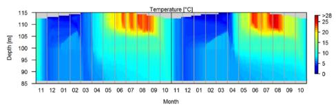
Figure 3: Modelled temperature distribution in the central basin with a groundwater inflow in the metalimnion (Var. 3) in the model years 2002 and 2003
