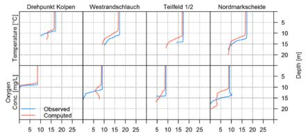
Figure 2: Observed and computed temperature and oxygen profiles in the reservoir Lohsa II
