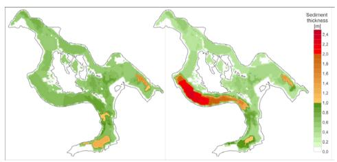
Figure 6: Projected thickness of the iron sediments in the reservoir Lohsa II after 20 years with a groundwater inflow near the surface (Var. 2, left) and in the metalimnion (Var. 3, right) of the central basin
