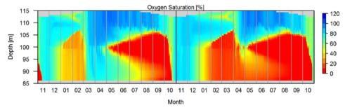
Figure 4: Modelled distribution of the oxygen saturation in the central basin with a groundwater inflow in the metalimnion (Var. 3) in the model years 2002 and 2003
