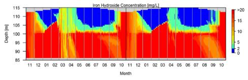
Figure 5: Modelled iron(III) hydroxide distribution in the central basin with a groundwater inflow in the metalimnion (Var. 3) in the model years 2002 and 2003
