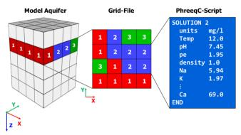
Figure 1: Assignment of PHREEQC scripts and the initial and boundary conditions to the cells of the multicomponent transport model using grid files
