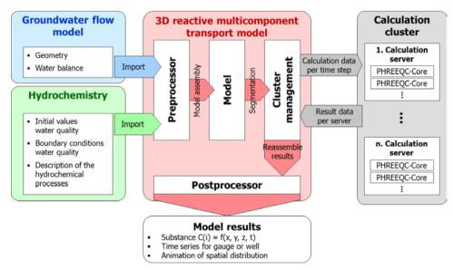
Figure 2: Structural scheme of the reactive multicomponent transport model
