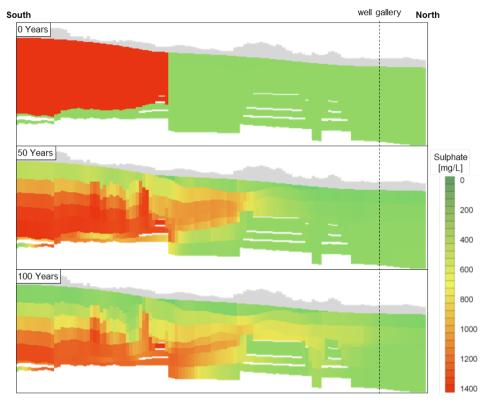
Figure 3: Distribution of the sulphate concentration in a vertical south-north section through the multicomponent transport model at the start of simulation (top), after 50 years (middle) and after 100 years (bottom)
