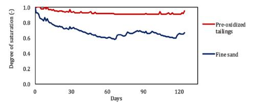
**Figure 5.** Variation of degree of saturation with time for both columns during modeling of field conditions with daily temperatures and precipitation values from Folldal from June to September.
