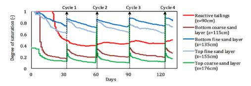
Figure 3. Variation of the degree of saturation with time for column 2. The elevation z of the sensors in the column is indicated (also see Figure 1).
