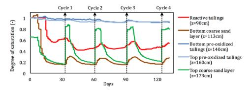
*Figure 2.* Variation of the degree of saturation with time for column 1. The elevation z of the sensors in the column is indicated (also see Figure 1).
