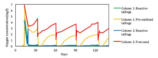
Figure 4. Variation of oxygen concentrations with time for both columns.
