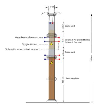
Figure 1: Column setup, showing location of the various sensors used to measure volumetric water content, pore pressure and oxygen concentrations.
