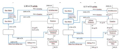
Figure 5 Simplified water balance calculations for conventional tailings (a, on the left) and for thickened tailings management (b, on the right)
