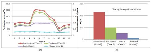
Figure 3: Risk related to seepages from tailings management facilities. Monthly fresh water make-up of the plant (a) and the estimated total seepage from the tailings facilities (b)
