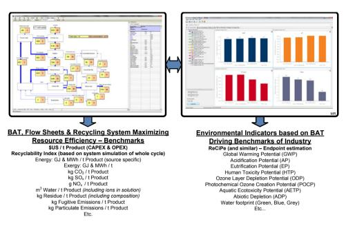
**Figure 1** Summary of the methodology: Left the HSC Simulation (www.outotec.com) of the water system for the four cases and right the environmental footprint calculation produced from the simulation results by life cycle assessment tool GaBi (www.thinkstep.com) (Reuter et al, 2015).
