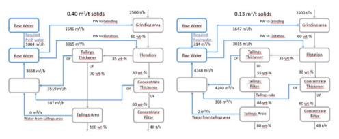
Figure 6 Simplified water balance calculations for paste thickening (a, on the left) and for filtered tailings management (b, on the right)
