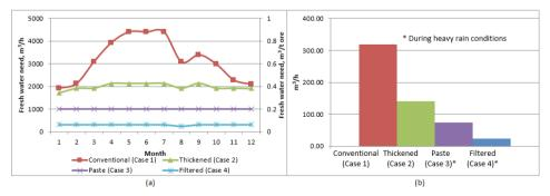
**Figure 4** Risk related to seepages from tailings management facilities at an arid region. Monthly fresh water make-up of the plant (a) and the estimated total seepage from the tailings facilities (b)
