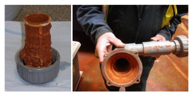
Figure 3 Blocked strainer filter on mine water feed to heat exchanger (left) and ochreous deposits on the heat exchanger inlet (right).
