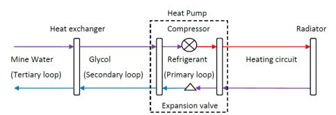
Figure 1 Schematic diagram of heat pump system installed at Dawdon
