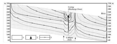
Figure 2 The scheme of groundwater movement after flooding (on the left – the surface watershed, the impermeable boundary; to the right – the river; the size of the block horizontally – 50 m, the number of layers – 10). 1 – grid layout; 2 – groundwater discharge into the caving; 3 – the direction of groundwater flow.
