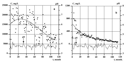
**Figure 1** Change in the content of components and pH in the groundwater of the discharge zone after flooding (solid line – polynomial approximation of the third degree): a - sulfate ion (R2 = 0.52), b - manganese (R2 = 0.74)
