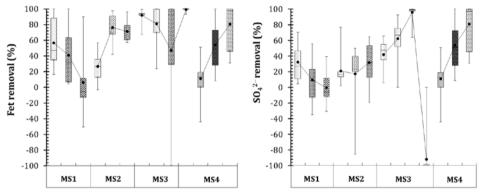
Figure 2 Relative removal of Fe and SO  $_{4}^{2-}$  (minimum, 25% percentile, median, 75% percentile, maximum, mean) during multi-step treatment of AMD
