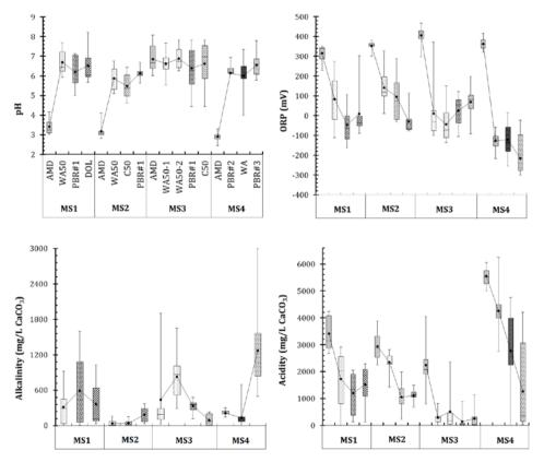
Figure 1 Physicochemical evolution of effluents in the columns during laboratory multi-step treatment of AMD (minimum, 25% percentile, median, 75% percentile, mean, maximum) AMD, WA50, PBR#1, PBR#2, PBR#3, DOL, C50, WA
