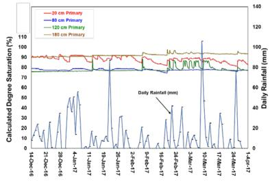
Figure 4 Calculated degree saturation at the WRSF2 monitoring location.
