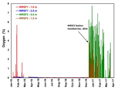
Figure 3 Oxygen concentration within the WRSF sealing layer.
