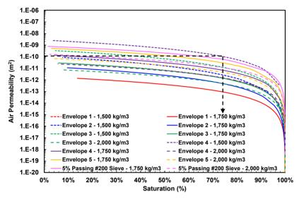
Figure 6 Air permeability of Martabe material under various levels of compaction.
