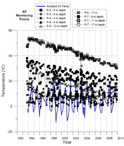
Figure 3 Temperature data with depth at the Equity Silver site (from Morin 2010).
