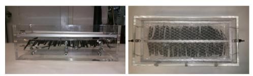
*Figure 1*: Images illustrating the LFCR design a) side view b) top view of the 8 L LFCR prior to inoculation fitted with strips of carbon microfibers, heat-exchange coil and harvesting mesh plate.
