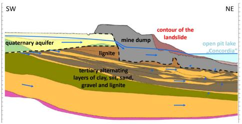
Figure 2 Cross section to show the complex geological and hydrogeological situation.
