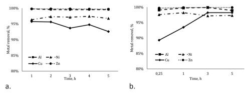
Figure 2 Metal removal efficiency by EC using iron electrodes at a. 1L reactor, b. 70L reactor (initial pH 6.4, æ 5.56 mS/cm, current density 12 mA/cm2)
