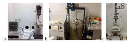
Figure 1 a. EC reactor 1L b. EC reactor 70 L c. Nutsche filter.
