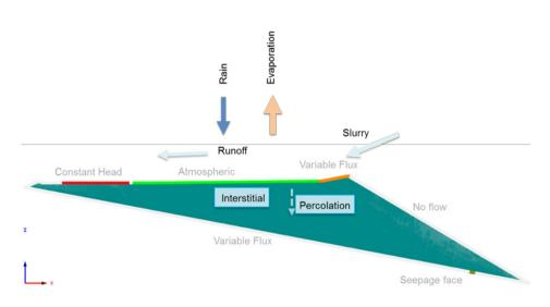
Figure 1 Illustrated processes and boundary conditions of the 2D simulated tailings dam
