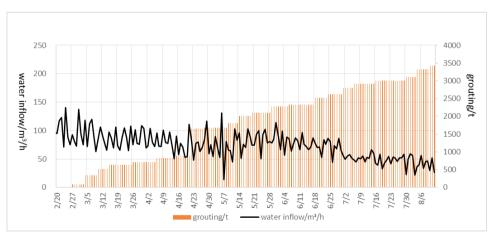
Figure 5 Mine water reduction during grouting process
