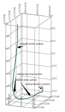
Figure 1 3-D directional well structure.
