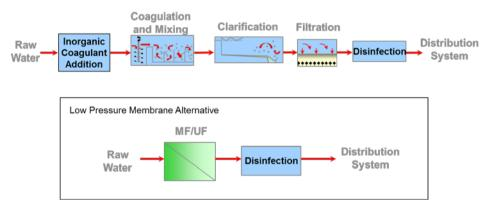
Figure 4 Membrane versus conventional process treatment
