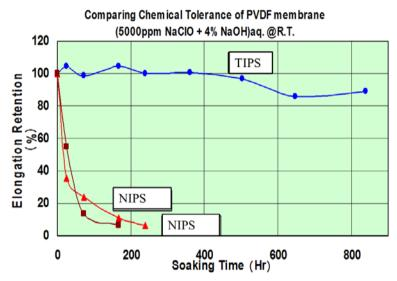
Figure 2 Chemical tolerance of differing manufacturing methods of PVDF membranes
