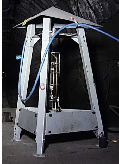
Figure 4 water measuring probe with frame
