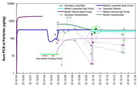
Figure 4 Measured values for the total PCB content of the particulate solid (= filterable substances) with calibration of the Boxmodel for three Saar pumping stations (Luisenthal, Viktoria, Camphausen).
