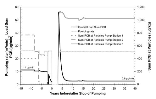
Figure 5 Model prognosis for the development of the PCB load as well as the determining pumping rates and PCB solids content for the total water extraction in the Saar model area.
