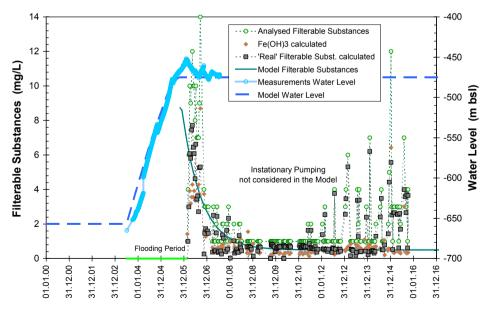
Figure 3 Measured values for particulate solids in mine water Camphausen with evaluations and calibration of the Boxmodel.
