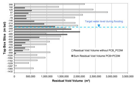
Figure 2 Depth distribution of the residual void volume from mining operations within and outside the period of use of PCB/PCDM-containing operating fluids (water province Duhamel / Ensdorf).
