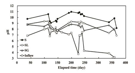
Figure 2 Inflow and outflow pH for the S, SL, and SG reactors as a function of elapsed time.
