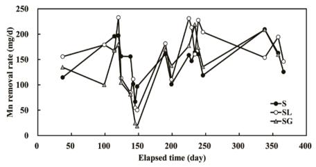
Figure 3 Mn removal rate at the outflow from the S, SL, and SG reactors as a function of elapsed time.
