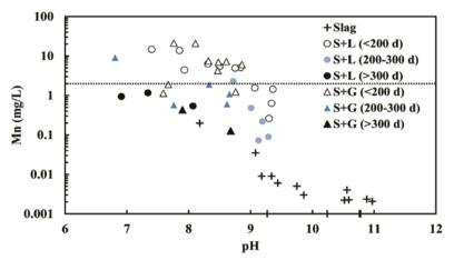
Figure 4 Variation in Mn concentrations with pH for specific reactions time periods for the S, SL, and SG reactors.
