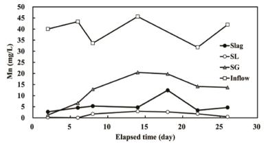
Figure 6 Variation in Mn concentrations as a function of elapsed time since Fe addition for the S, SL, and SG reactors.
