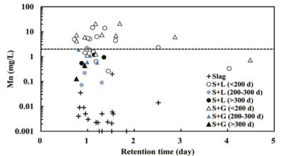
Figure 5 Variation in Mn concentrations with retention time for specific reaction time periods for the S, SL, and SG reactors.
