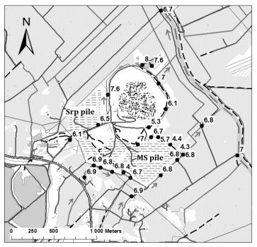
*Figure 2* pH values measured in the surface waters around the Hitura mine site in June 2016. SRP pile = serpentinite pile, MS pile = mica schist pile (Basemap © National Land Survey of Finland.)
