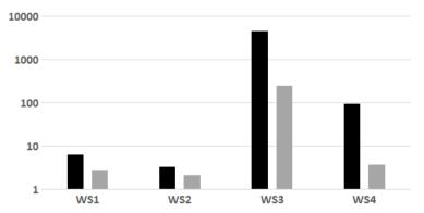
Figure 3 Dissolved Ni and Cu concentrations in the Hituranoja and Töllinoja ditches in the background sampling points (WS1 and WS2), seepage point (WS3) and in the ditch downstream of the mica schist waste rock area (WS4).
