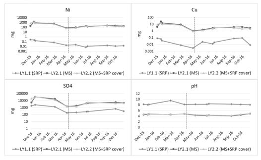
**Figure 4** Amounts (mg) of Ni, Cu and SO4, and pH leached out of the lysimeters during the observations period. LY1.1 = serpentinite, LY2.1 = mica schist, LY2.2 = mica schist with 15 cm of serpentinite on top. The dashed line represents the date when LY2.2 was covered with a 15 cm layer of serpentinite.
