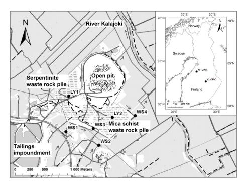
Figure 1 The location and setting of the Hitura mine site and sampling points. WS = water sampling point, LY = sampling point for lysimeter tests. (Basemaps © National Land Survey of Finland.)
