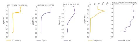
Figure 11: Water column profiles for Pit Lake A (Jan 2017).
