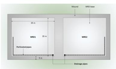
*Figure 1* Dimensions of the basal area of waste rock deposit with drainage. Light gray surface is the inner area, while the dark grey borders are the berms.WRD1 = south dump, WRD2 = north dump.
