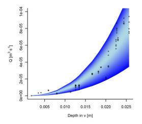
*Figure 2* Rating curve for discharge from the north waste rock dump. Lighter blue indicates the lowest absolute sum of residuals, i.e. the best fit to data, while the darker blue is a poorer fit.
