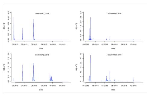
Figure 3 Leachate discharge from north and south waste rock dumps, calculated from rating curves and measured water levels. Note that discharge scales are different for each diagram.
