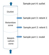
Figure 1: schematic diagram of the column experiment
