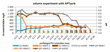
**Figure 3**: pH development and copper concentration for each column zone for the column experiment with APTsorb as reactive material in the retention zone vs. exchanged pore volumes (PV) of the zone
