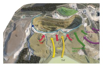
Figure 1 Conceptual flow model contributing to drainage collection channel.
