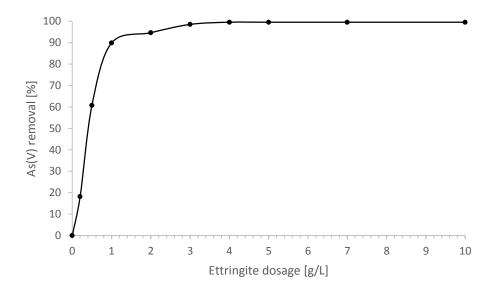
**Figure 1** The effect of sorbent dosage on the sorption of arsenate on ettringite. Initial As(V) concentration = 1.7 mg/L, ettringite dosage = 0—10 g/L, temperature =  $20 \pm 2$  °C, agitation = 250 rpm, contact time = 24h, and solution volume = 25 mL. Values are presented as the average of duplicate experiments.
