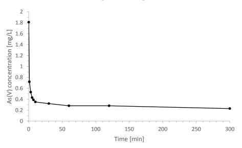
**Figure 3** The effect of contact time on the sorption of arsenate from a model solution on ettringite. Initial arsenate concentration = 1.8 mg/L, ettringite dosage = 1 g/L, temperature =  $20 \pm 2 \text{ °C}$ , initial solution volume = 1 L, stirring 250 rpm, and samples taken between 0-5 h.
