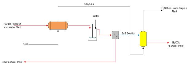
Figure 4 The chemical recovery process
