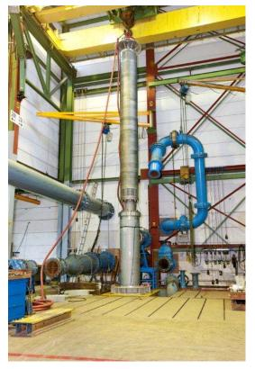
*Figure 1*: A Ritz HMD pump being placed in the test bay. Note the two suctions to combat axial thrust.
