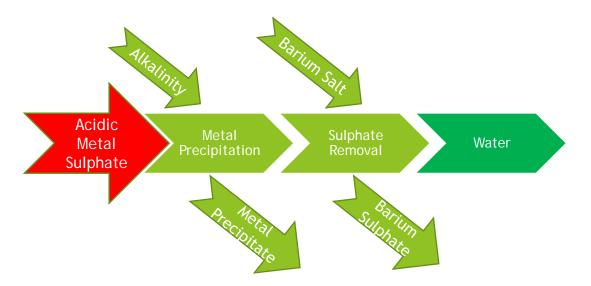
Figure 3 The ABC water treatment process concept
