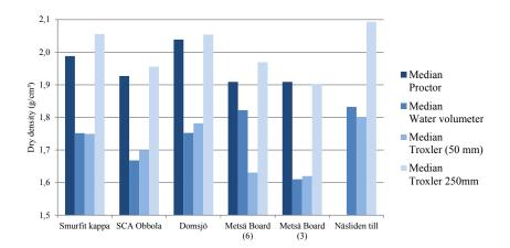
*Figure 4* Dry density of a till and a mixture of till and 10 % of GLD from different paper mills compacted in the laboratory using a Proctor hand hammer and in the field using a hydraulic plate compactor. The field samples were analyzed with both a water volumeter and Troxler apparatus.
