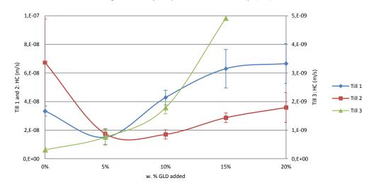
Figure 3 Hydraulic conductivity (HC) of the different mixtures. Note that the HC for till 3 is on the right y-axis.
