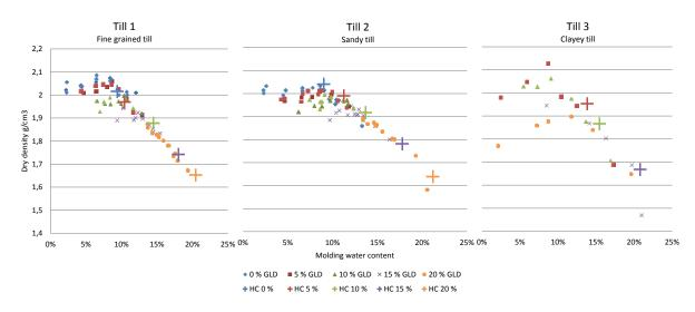
Figure 2 Proctor compaction curves, with dry density (g/cm<sup>3</sup>) plotted towards molding water content of the different tills and till-GLD mixtures. The pure tills are plotted with blue rhombs, 5 w. % GLD-mixtures in red squares, 10 w. % GLD-mixtures in green triangles, 15 w. % GLD-mixtures in purple crosses and 20 w. % GLD-mixtures in orange dots. The plus-marks represent the estimated dry density and molding water content of the samples tested for hydraulic conductivity (HC).
