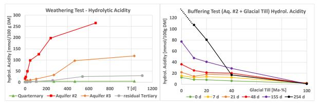
*Figure 2*: Hydrolytic Acidity in Weathering Tests of different Investigation Units (left) and Buffering Tests Aquifer #2 + Glacial Till (right) [3], [4]
