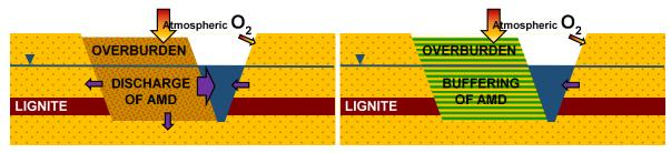
Figure 1: uncontrolled discharge from AMD (left) or structured buffering (right) in lignite opencast [4]
