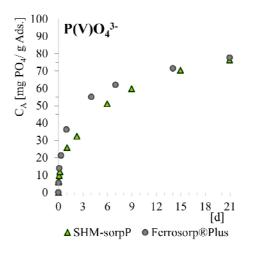
Figure 3 Adsorption behaviour of phosphate
