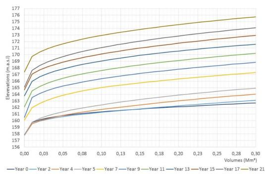
Figure 1 Examples of a set of stage storage curves for a fictive tailings storage facility. Own elaboration.
