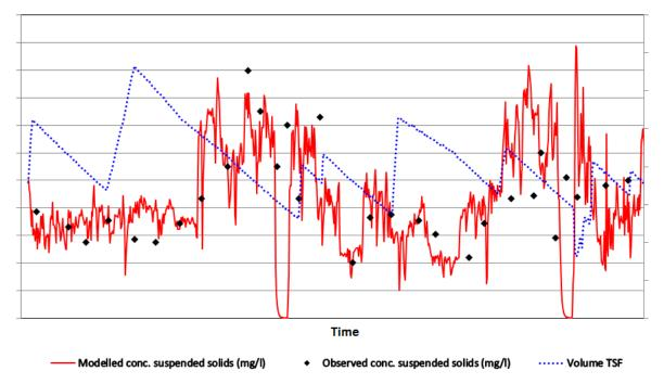
Concentration of suspended solids in effluent water from clarification pond, modelled and observed
