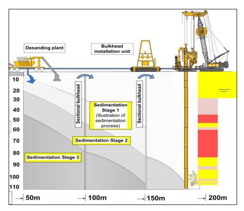
Figure 2: Pile guided Trench Cutter Cut-off wall systems
