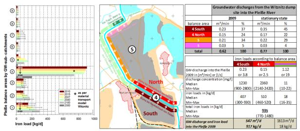
Figure 2 Projection results of iron loads entering the Pleiße from the balance areas 1 to 9 in 2010, 2015, 2027, 2040, 2100, 2300 (\*as per material transport model Witznitz) (left) (IBGW and Ecosystem Saxonia 2011); Baseline balances of groundwater flow and iron loads entering the Pleiße from the Witznitz dump site between the mouth of the Wyhra and the Trachenauer Weir (right) (IBGW 2009b)
