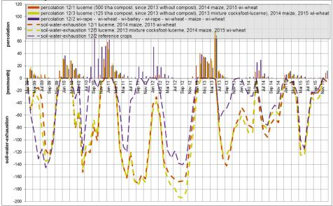
Diagram 1 Lysimeter results of soil-water exhaustion and quantity of percolation per month 2009 - 2015, Comparison of lucerne, cocksfoot/lucerne and reference crops (GFI 2015)
