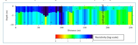
Figure 3: Measured and modelled two layer resistivity profile over a leakage channel.
