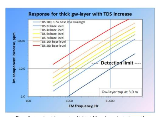
Figure 2: a) used model parameters, b) detectability of groundwater layer with increasing salinities over EMI frequencies.
