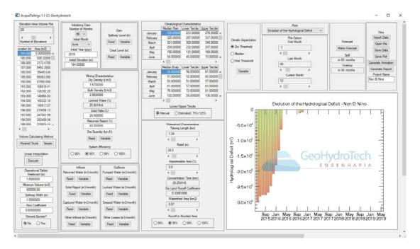
Figure 1 Screen Capture of the AcquaTailings Graphics User Interface.
