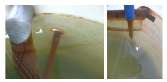
Figure 2 Photographs of iron hydroxide coatings formed downstream the sand filter from the filtrate
